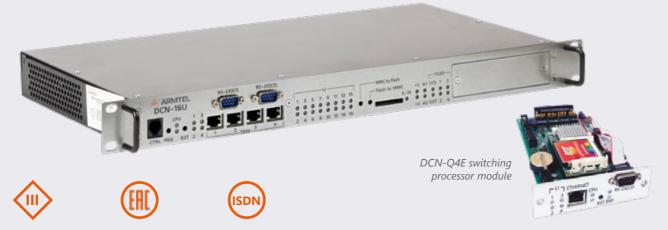
DCN-16U digital subscribers exchange unit is designed for operation as a part of DCN digital Intercom and PA/GA system on the basis of DCN-2 or DCN-Q4E switching processor module and provides for interfacing with digital subscriber equipment by  $Uk_0$ -interface. DCN-16U transmits digital data between 15 subscriber  $Uk_0$ -interfaces and E1 line of a central exchange unit. In addition, there is a version of DCN-16U with built-in DCN-Q4E switching processor module.
