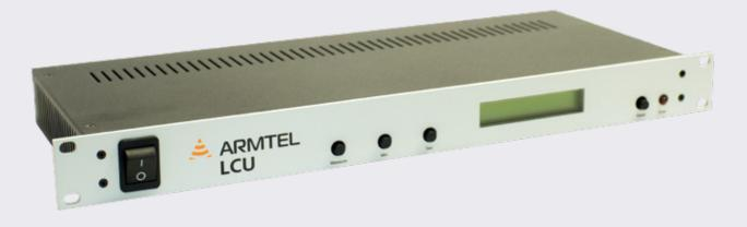
The ARMTEL LCU Line Monitoring Module is a digital speaker line monitoring system to monitor ground faults and short circuits, impedance deviations and line breaks in 100 V loudspeaker lines.
